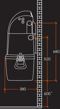
\* Minimum space recommended to allow the dust container to be emptied comfortably.
